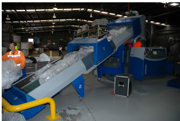
Right: The new Erema extruder – the latest technology in plastic recycling and the only one of its kind in Australasia
